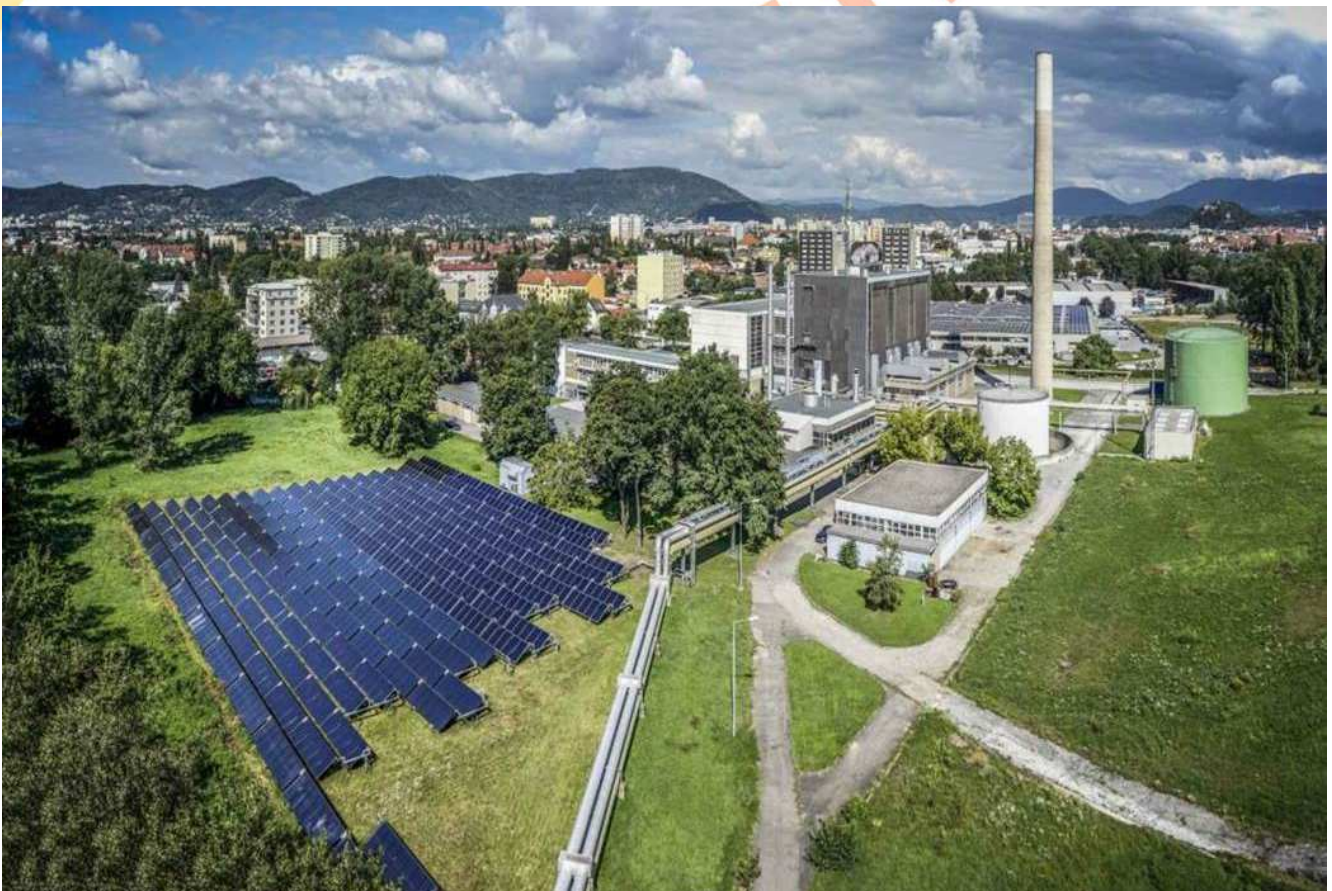
Test field of 2500 m 2 located in Graz for different solar collector's testing and selection of most suitable one for the large scale solar plant to be built in Kremsmünster. Source: Solid
